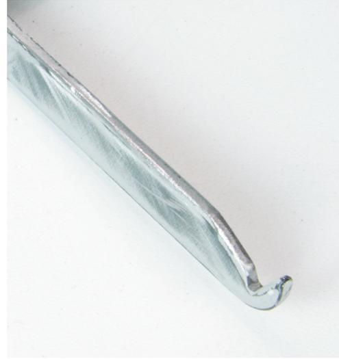
Grind overspray off of hook (grind down to bare metal).
