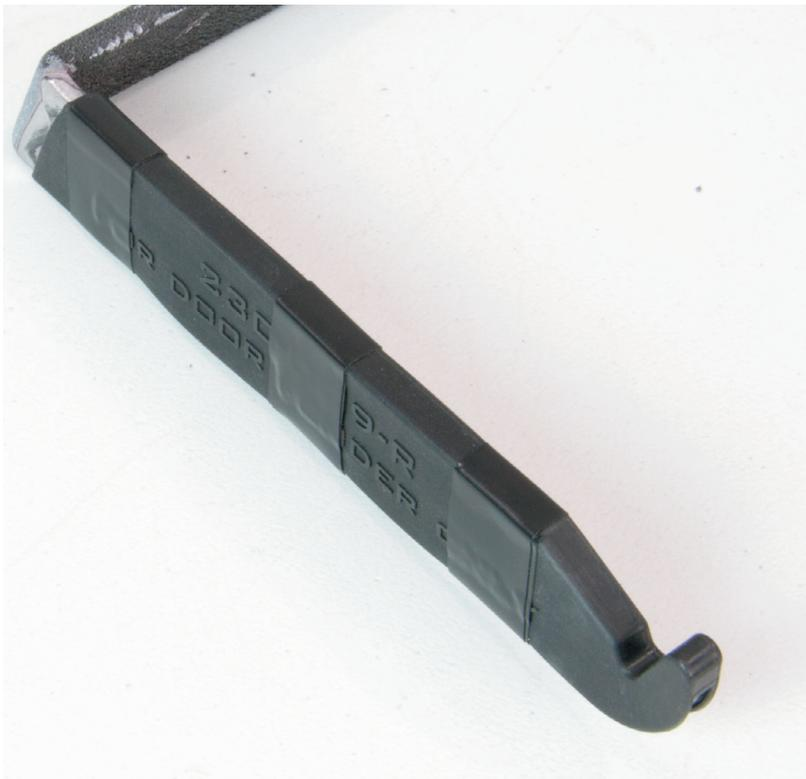
Slide rubber sleeve onto hook and apply electrical tape as shown to secure sleeve onto hook. When overspray gets excessive, cut tape along bottom edge and replace with new sleeve.
