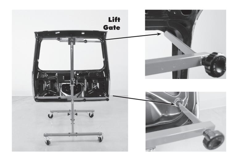
Tailgate mounting: remove right and left upper Support Arms from upper Tee Frame Tube (P/N 220-007). Rotate Support Arm hooks a quarter turn downward, re-insert 5 inches into upper Tee Frame Tube. Securely tighten upper Tee Frame Tube Hand Knobs. Insert right and left Extension Arms (P/N 220-010 and P/N 220-011) into upper right and left Support Arms. Center tailgate, securely tighten upper Support Arm Hand Knobs (see photo 3).
