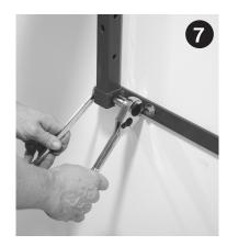
Tighten side rail bolts using 9/16" socket and 9/16" end wrench.
