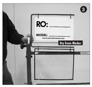
Set RO Holder onto RO Bracket and tighten hand knob to any desired location. Insert dry erase marker as shown into RO Bracket.
