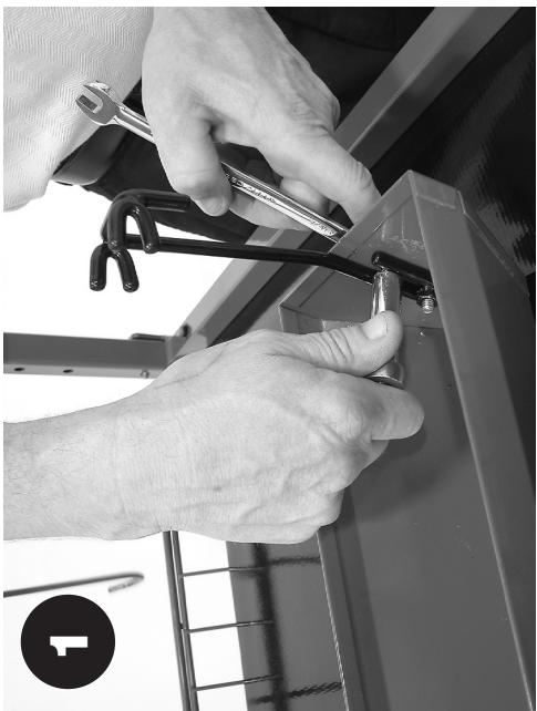
Install Pan Hooks using supplied 1/4" nut, bolt and washer. Note: both V-hooks point in the same direction.
