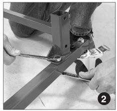
Bolt leg support tubes to lower frame support. If you want to nest the SuperStorage Parts Cart, move leg support to outward position.
