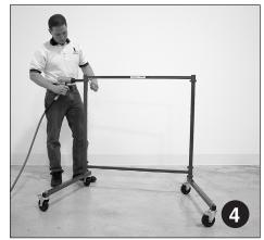
Install upper frame support, then tighten all bolts.
