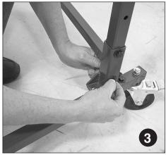
Slide side rail tube into lower base support. Insert bolts. *Note: do not tighten bolts until frame is completed.*
