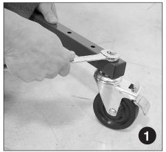
Install wheels to leg support tubes.
