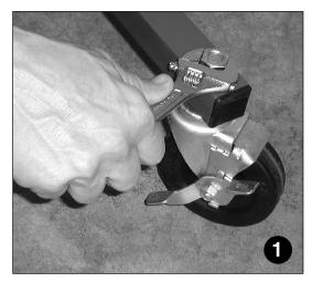
Install wheels to leg support tubes.
