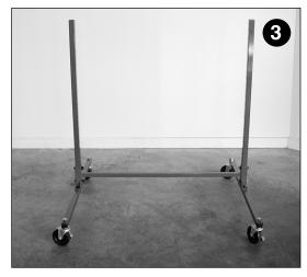
Slide longer side rail tubes (P/N 290-005) into lower base support, insert bolts. *Note:* do not tighten bolts until frame is completed.
