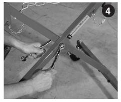
Connect frame support tubes using 3/8" x 3/4" bolt and nylon lock nut. Note: use flat washer between frame support tubes. Do not overtighten.
