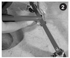
Use 3/8" bolts to connect lower support tube to frame support tube. Tighten firmly with 9/16" wrench.
