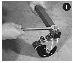
Insert wheels, tighten with 3/4" hand wrench.
