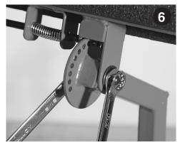
Install panel rest assembly using 3/8" shoulder bolt with two flat washers on each end and nylon lock nut. Note: do not overtighten.
