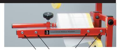
**Step one:** Remove four screws using a 5/16 inch socket
