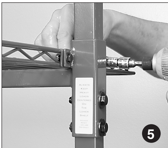
Install Shelves using 1/4" bolt with flat washer on outer side and 1/4" lock nut on inside. After assembly is complete, fully tighten all bolts.
