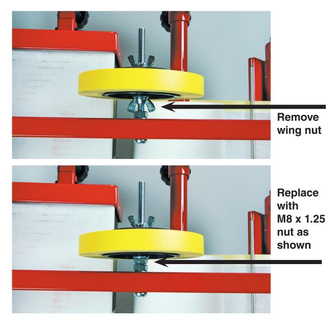
If you use metric paper, which is narrower than standard paper, replace wing nut as shown in above photo.
