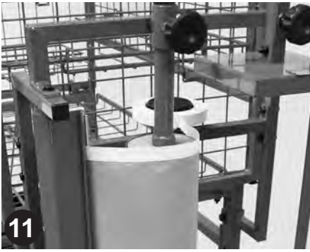
Tape hub assembly showing paper and tape direction. Use downward pressure on Upper Paper Support to adjust how easy paper unrolls.
