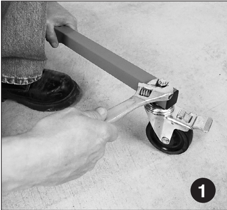
1 Install Total Lock Caster Wheels. Secure to Support Tubes P/N 220-001.
