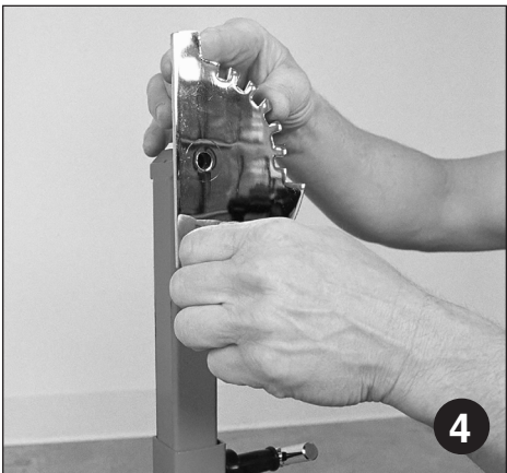
4 Slide Inside Frame Post (P/N 220-004) into Frame post. Install Index Plate lower bolt (finger-tight only).
